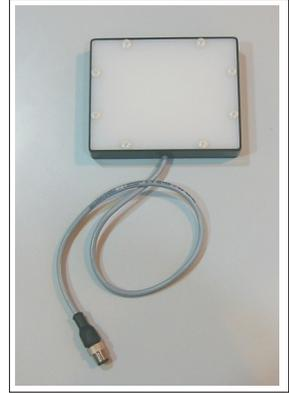
The connection cable, coated with PUR, is 30 cm long and terminated by an M-12 male connector. The "M" version has a pin which permits to adjust the luminosity using a voltage-controlled analog signal from 0 to 10V.
